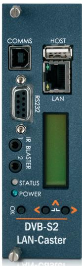
Use the front panel LCD and push buttons to set the IP address settings.
