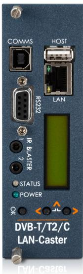
Use the front panel LCD and push buttons to set the IP address settings.
