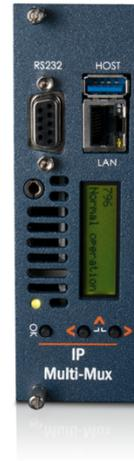
The 796 IP Multi-Mux is an IP network gateway device that provides a secure interface between an IPTV service provider's IP delivery network and a customer's internal network.
