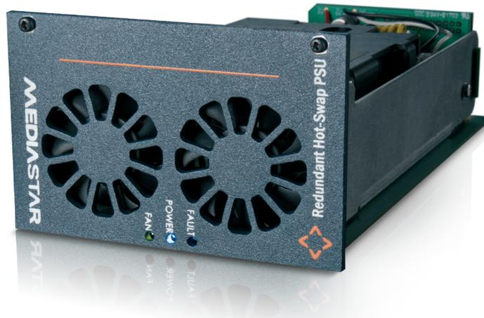
The 726 power supply module is designed for use in the dual redundant MediaStar 770-DR rack only. This rack has two independent 726 PSU modules, each individually capable of powering the entire rack so in the event of a PSU failure, the other power supply will automatically take over without disruption of the 'blade' processor modules.
